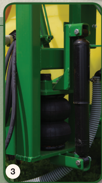
3. Airbag and shock absorber suspension
